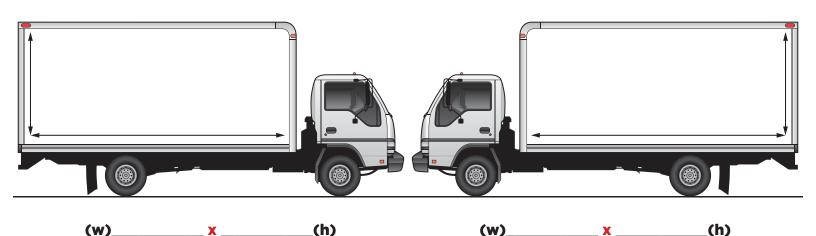
**SIDE PANELS: WIDTH MEASUREMENT** from the front radius panel to the front of the rear post. HEIGHT MEASUREMENT from bottom of the upper rail to top of the bottom rail.
